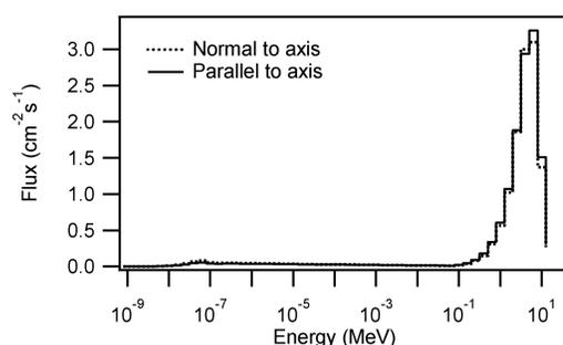
Isotropic angular response of the NNS demonstrated through measurements of AmBe neutrons with detector in two orientations.
