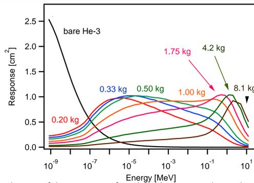
The shapes of the response functions (or energy dependent neutron counting efficiencies) are similar in appearance to those of the BSS. The increasing HDPE mass is as follows: 0 kg (bare detector) and 0.2, 0.33, 0.50, 1.0, 1.75, 4.2 and 8.1 kg.
