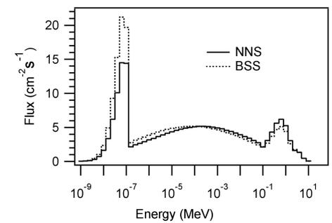
NNS and BSS measured neutron energy distributions at the Basement Perimeter Wall (BPW) at the Gentilly 2 (G2) CANDU nuclear power reactor. NNS and BSS were at slightly different locations.
