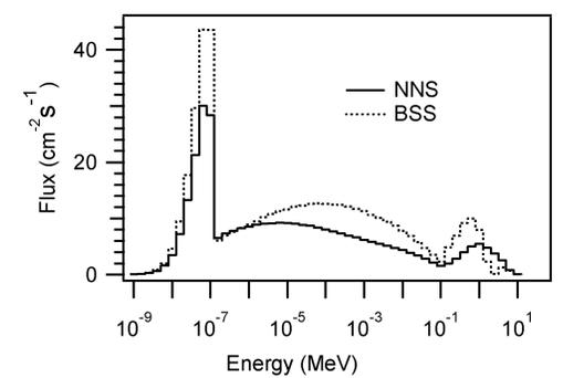
NNS and BSS measured neutron energy distributions inside the Heat Transport Assembly Room (HTAR) at the Gentilly 2 (G2) CANDU nuclear power reactor. NNS and BSS were at slightly different locations.
