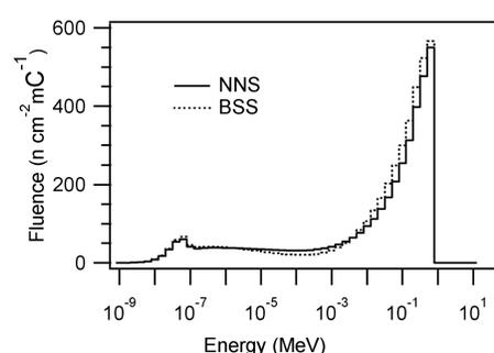
Spectrum measured for neutrons produced by the <sup>7</sup>Li(p,n)<sup>7</sup>Be reaction on thick Li targets. The measurements were performed at the 3MV KN accelerator facility at McMaster University. The maximum neutron energy was 510 keV in this case..
