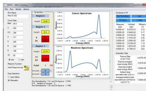
In a given field, 8 measurements are performed with the 8 configurations of the HDPE. The unfolding process creates an energy distribution over 52 energy bins. This requires a dedicated unfolding code. To this aim, we produced a Graphical User Interface over the Stay'SL least square minimization algorithm [4].
