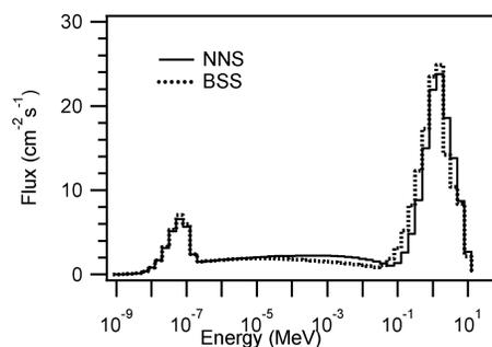
BSS and NNS spectra measured for bare <sup>252</sup>Cf at the AECL Chalk River Neutron Irradiation Facility (high scatter condition).
