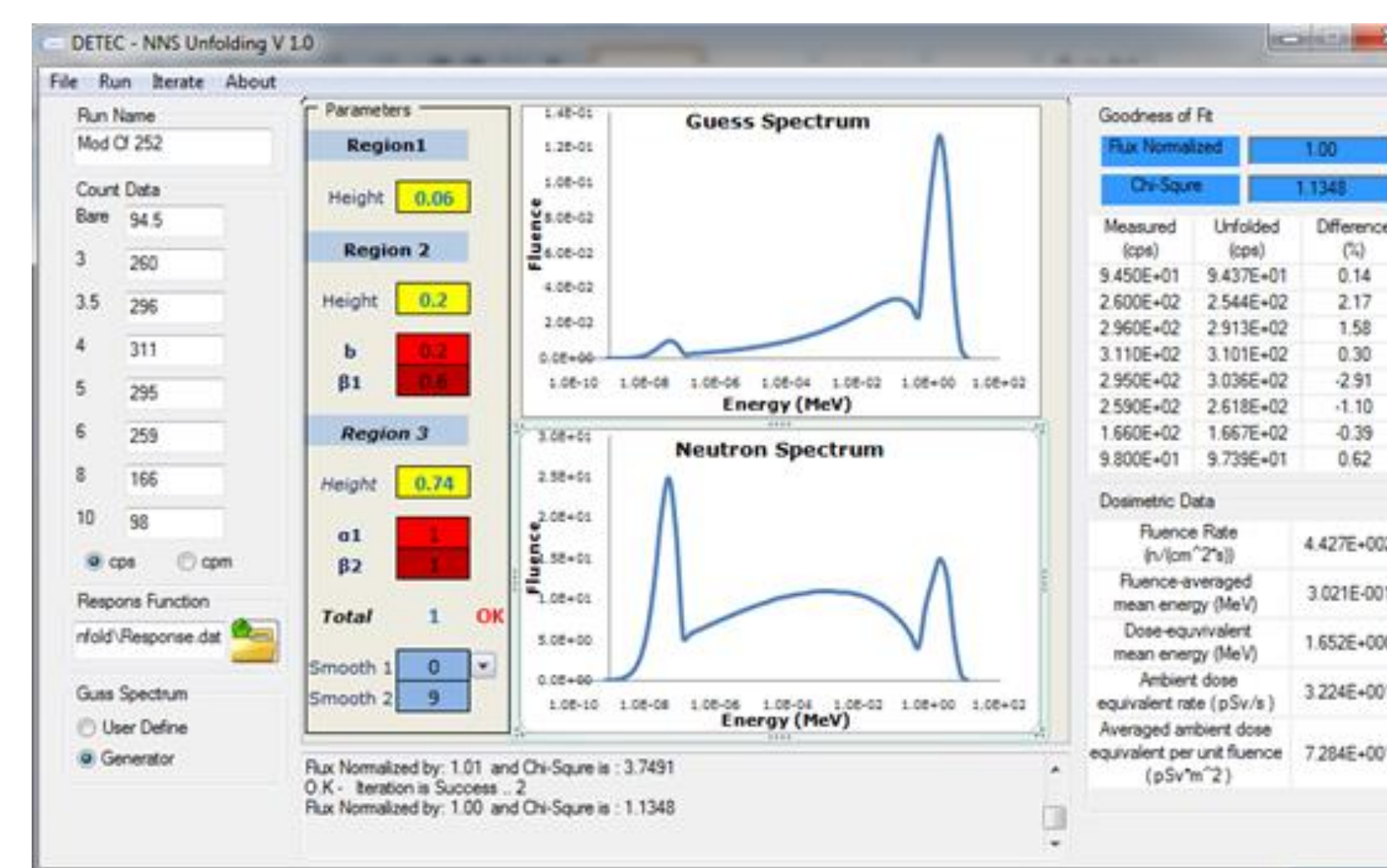
Figure 4: Screen shot of the graphical user interface of the unfolding software. It requires a guess solution provided by the user and uses a mean square minimization algorithm.
