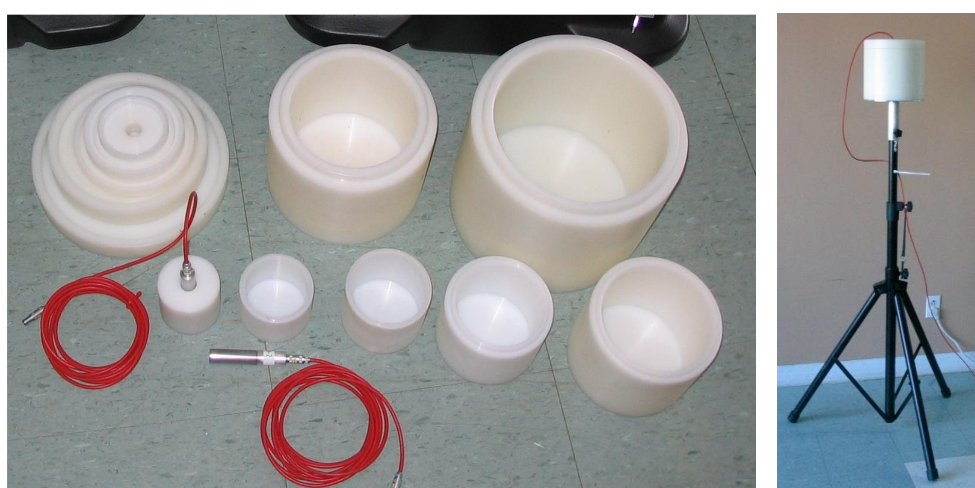
Figure 1: NNS fully disassembled (left) and ready for use on a tripod (right). The small cylindrical 3 He counter is shown.
